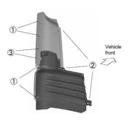
When removing or reinstalling the corner panel, be very careful not to allow the front end of the door to touch and damage the corner panel when the door is opened or closed.
